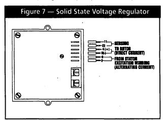
The voltage regulator also incorporates a "voltage surge protection circuit." This circuit prevents troublesome surges in the generator AC output voltage. Voltage surge is a common cause of damage to electronic equipment.
